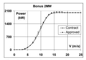
Figure 6: Power curve for the 2 MW turbines. Production figures can be found on www.middelgrund.com. The information is updated every 10 minutes
